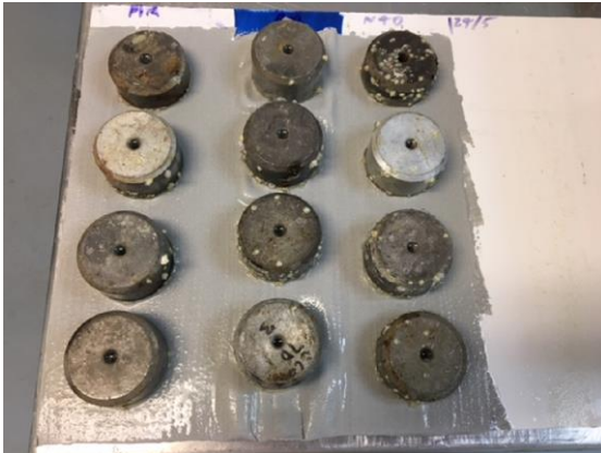
Wet bond testing of membrane. Picture 5:
